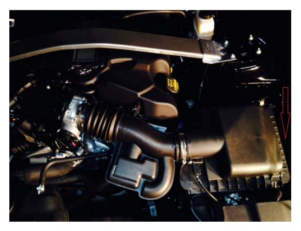
5. Remove the factory air box grommets and install into the new Cold Air Dam.
