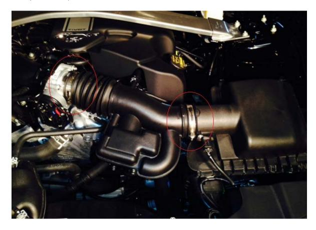
3. Disconnect Mass Air Flow sensor. The picture below shows the underside of the harness (detached). Use a flat head screw driver to pull the red tab and the harness pulls off easily.
