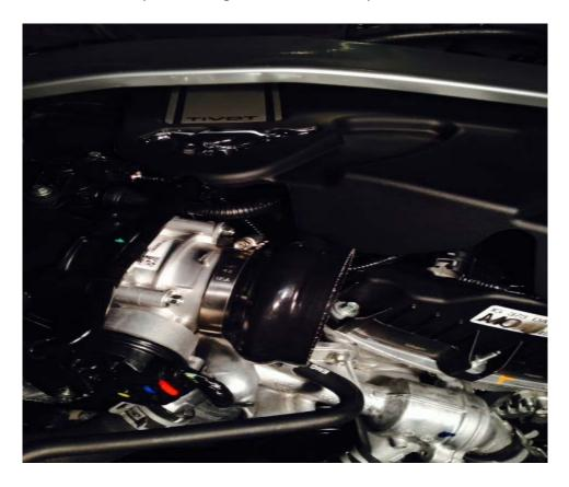
10. The other end of the new intake tube will attach to the new air dam with the supplied 2 1/4" 20 x 1/2" Button Head Bolts and 1/4" Flat Washers.
