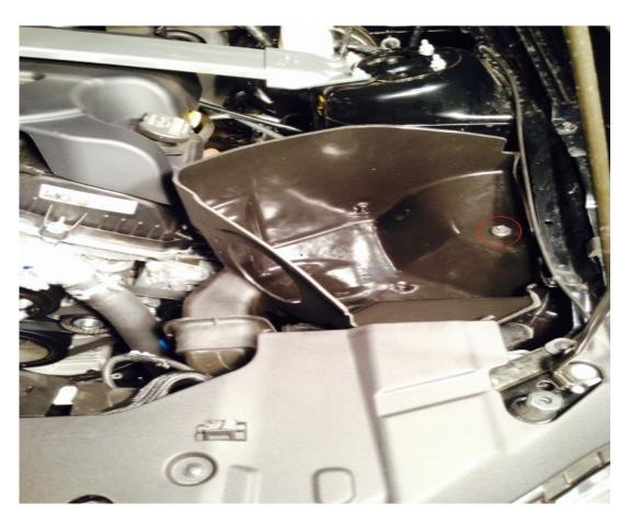
7. Remove the mass air sensor from the factory air box using the supplied #20 Torx Bit. Reinstall on the new intake tube using the supplied 8-32 Button Head Bolts. Note the position of the arrow on the mass air sensor.
