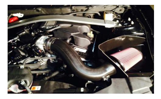
12. Tighten all your clamps down securely. Reinstall the mass air flow harness to the mass air flow sensor. Lastly, install the weather stripping around the new airbox and add your Roush decal.
