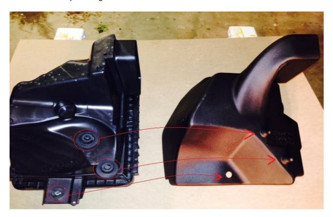
6. The new Cold Air Dam is now ready to be installed into the factory location. Using the old bolt, fasten the new Air Dam to the left fender.
