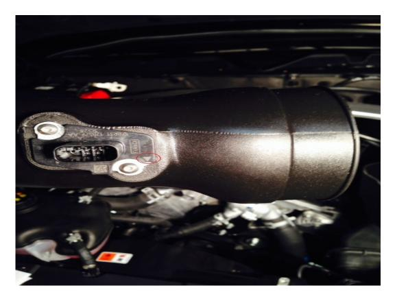
8. On the other end of the new intake tube install the supplied 5/8" Grommet and 5/8" Aluminum Fitting as well as the plastic 1/4" Fitting (Automatic Transmissions) or 1/4" plastic Plug (Manual Transmission).
