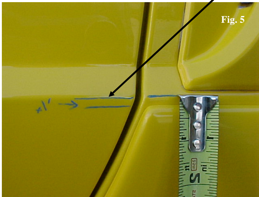
Fig. 4& 5: Install Rocker's 1/4" below body contour line.
