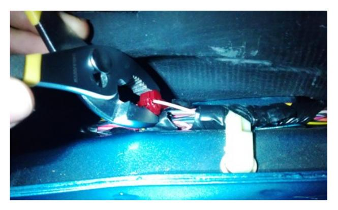
10. Finish routing the red wire down to the skid plate and plug it into the red wire tap. Tuck it in behind the kick panel so that it is out of view.
