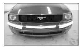
**13.)** Place the bumper over the inserts and locate using light pressure as shown below. Be sure all 6 tabs are accessible. Be sure that the bumper is centered on the vehicle.
