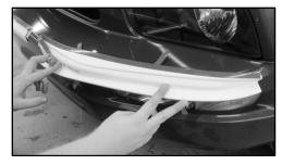
9.) Hold down insert D8 (or D6) in the center and pull the top two tabs toward the outside of the insert as shown below. Apply light pressure to the insert where the lining has been removed.
