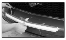
**5.)** Pull the bottom two tabs toward the outside of the vehicle as shown below. Apply light pressure to the insert where the lining has been removed.
