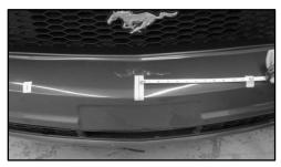
3.) Place insert C8 (or C6 for V6 Applications) on the center of the fascia as shown below. Be sure that all 4 inside tabs are accessible. Use light pressure to locate the part on fascia. Insert should fit snug against the fascia surface. Outside edges of the insert should be aligned with marks made in step 2.
