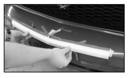
4.) Once insert is located, hold down the insert in the center and pull the top two inside tabs toward the outside of the vehicle as shown below. Apply light pressure to the insert where the lining has been removed.
