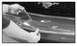
15.) Push the ends of the bumper in close to the body and pull the top two outer tabs toward the outside of the vehicle as shown below. Apply light pressure to the bumper where the lining has been removed.
