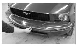
14.) With the bumper centered on the vehicle pull the top two center tabs toward the outside of the vehicle as shown below. Apply light pressure to the bumper where the lining has been removed.
