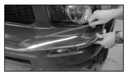
16.) Pull the bottom two tabs toward the outside of the body as shown below. Apply light pressure to the bumper where the lining has been removed.
