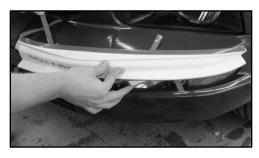
10.) Pull the bottom two tabs toward the outside of the insert as shown below. Apply light pressure to the insert where the lining has been removed.
