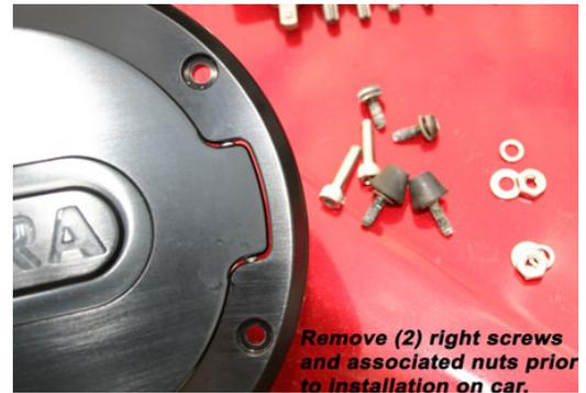
**Remove (2) right screws and associated nuts prior to installation on car.**
