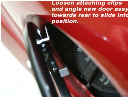
**Loosen attaching clips and angle new door assy towards rear to slide into position.**
