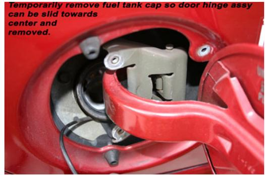
**Temporarily remove fuel tank cap so door hinge assy can be slid towards center and removed.**
