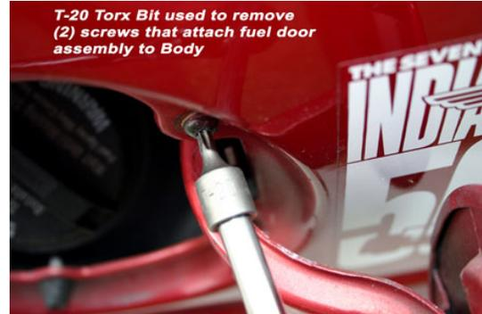
**T-20 Torx Bit used to remove (2) screws that attach fuel door assembly to Body**
