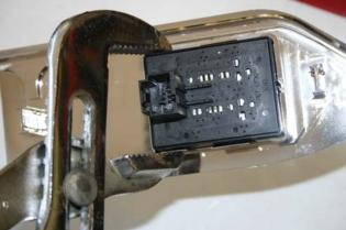
6. Using a small screwdriver or prying tool, remove the spring clips from the posts on the original door switch plate and transfer to the new switch plate. Install the new switch plate into the lower cover. Reconnect the wiring for the switches, temporarily turn the key to the on (but not start) position and test switches. If everything works well, reinstall on the door, using the alignment pins on the lower cover as a guide.
