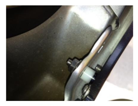
8. Use the 3/8" combination wrench to tighten each of the back bolts and locking in the alignment.
