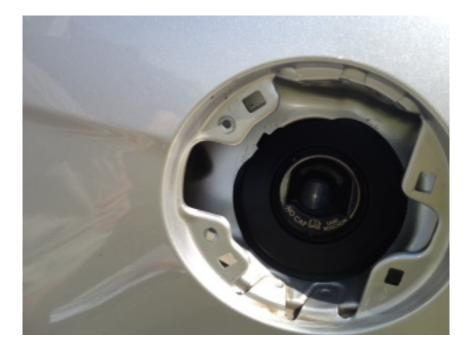
7. Remove the nuts and top spacer from the new fuel door, but leave the bottom spacer on it. The top right bolt only has a stud on it, which is not to be removed. Open the door to get the proper alignment and put it on the car by placing the bolts into the corresponding holes. Reach around the back and place the spacer then the nut on each bolt. Hand-tighten each one.
