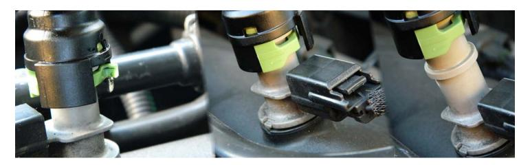
**4.)** Proceed to release "Quick Disconnects" tabs on throttle body intake.
