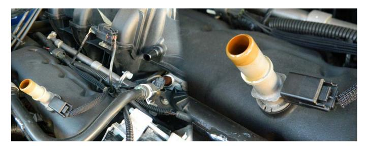
**5.)** Install JLT Oil Separator. 90 Degree Elbow clicks on (PCV) valve. Straight connector to throttle intake manifold. (You will hear a click when it's locked in place.)
