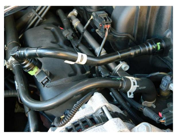
**3.)** Start with (PVC) side press green "Quick Disconnects" tabs to release hose. Slowly wiggle and pull off. If tabs are stuck you may require a small flat head screw driver. (Be very careful these are plastic clips do not apply too much pressure take your time.)
