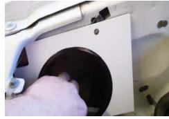
Install 45° Rubber elbow and clamps on to the JLT tube. There is a SHORT side on the elbow, be sure to put the SHORT side on the tube (part# should NOT BE SEEN). Insert round end into the hole in the apron plate and rotate it down and on to the throttle body. Tighten the clamp at the throttle body and leave the clamp on the tube loose for final adjustment.
