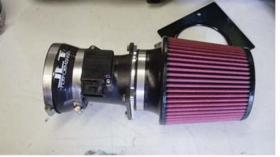
Put some tape around the hole in the apron. This will help prevent scratching the pipe during install. Bolt Apron Plate up using the stock air box bolt.
