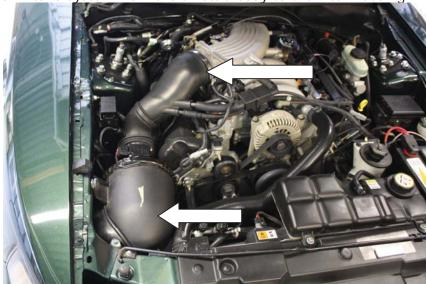
5 PULL the Inlet Air Temperature sensor from your stock inlet and install in the grommet on bottom side of JLT tube.
