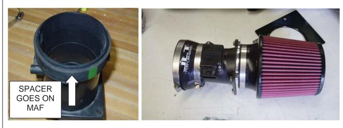
Unplug the hold down in the large wire harness where the MAF wire ties into it and pull toward the hole. Feed your MAF wires into the hole in the apron. You only need a few inches in there. Put some tape around the hole in the apron. This will help prevent scratching the pipe during install. Bolt Apron Plate up using the stock air box bolt.
