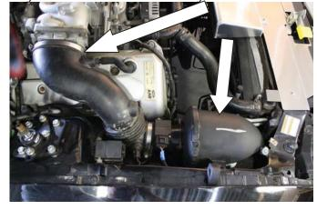
Unbolt your Mass Air Flow Sensor from the filter housing, and install the MAF filter adaptor using the supplied MAF gasket and bolts shown below. **Do not reuse the screen BOLTS GO THROUGH MAF AND THREAD INTO ADAPTOR**.
