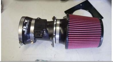
**7** PULL the Inlet Air Temperature sensor from your stock inlet and install the grommet in bottom side of JLT tube.
