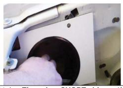
Install 45° Rubber elbow and clamps onto the JLT tube. There is a SHORT side on the elbow, be sure to put the SHORT side on the tube (the part# should NOT BE SEEN). Insert round end into the hole in the apron plate and rotate it down and onto the throttle body. Tighten the clamp at the throttle body and leave the clamp on the tube loose for final adjustment.
