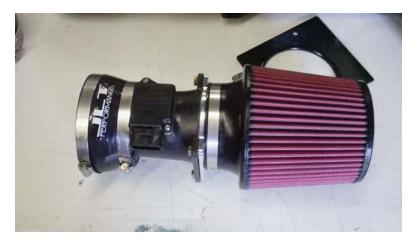
**7** PULL the Inlet Air Temperature sensor from your stock inlet and install in the grommet on bottom side of JLT tube.
