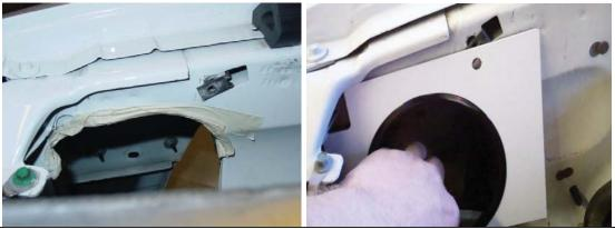
Install coupler and clamps on to the JLT tube, then insert round end into the hole in the apron plate and rotate it down and on to the throttle body. Tighten the clamp at the throttle body and leave the clamp on the tube loose for final adjustment.
