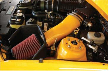
This kit includes an S&B Powerstack pre-oiled reusable air filter. The frequency you should clean your filter will depend on your driving conditions. It is recommended to check your filter at every oil change or 3,000 miles. If there is a build up of dirt as thick as the wire mesh, then it's time to clean your filter. As dirt builds up on your filter, the restriction of the airflow also increases. More frequent cleanings will improve your fuel economy and your vehicle's performance.
