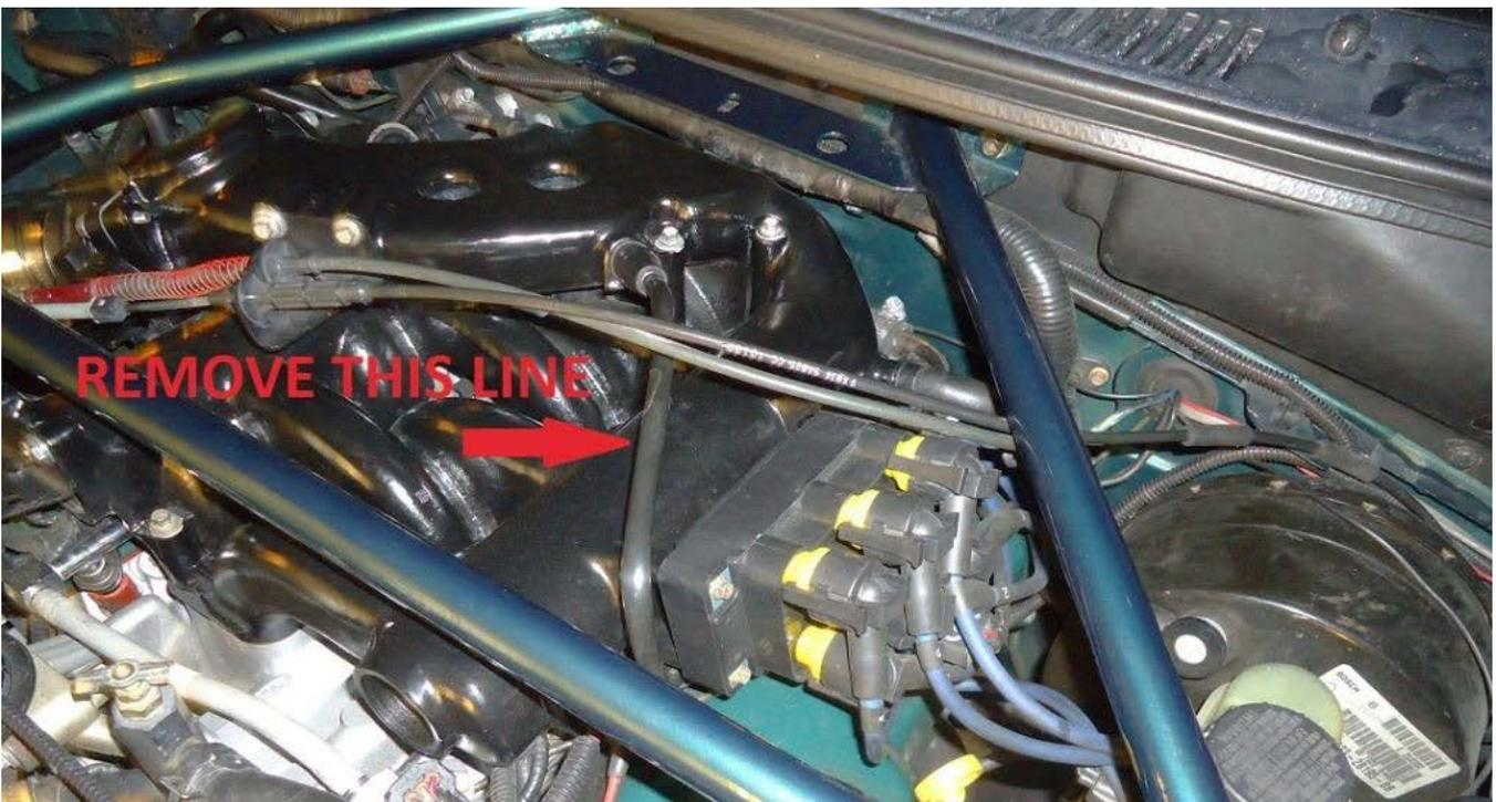
2. **For non-Cobra models:** Cut the hard line just before the bend on each end as shown.
