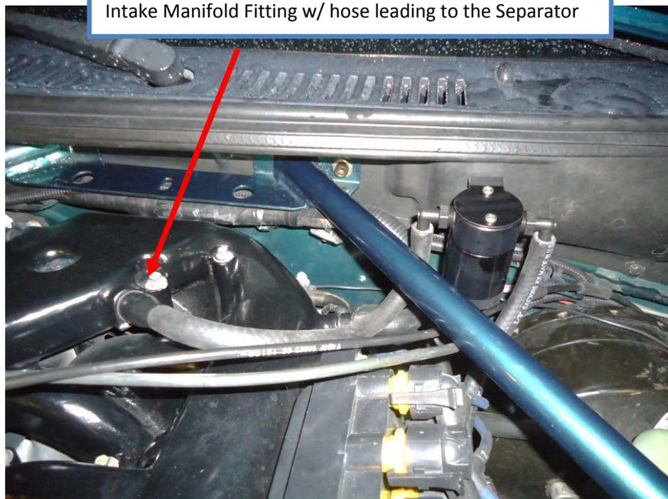
10. **For Cobra ONLY:** Remove the PCV connection from the PCV valve and install the supplied JLT hose in its place. Install the other end of the new hose to the right side of the oil separator. Trim excess.
