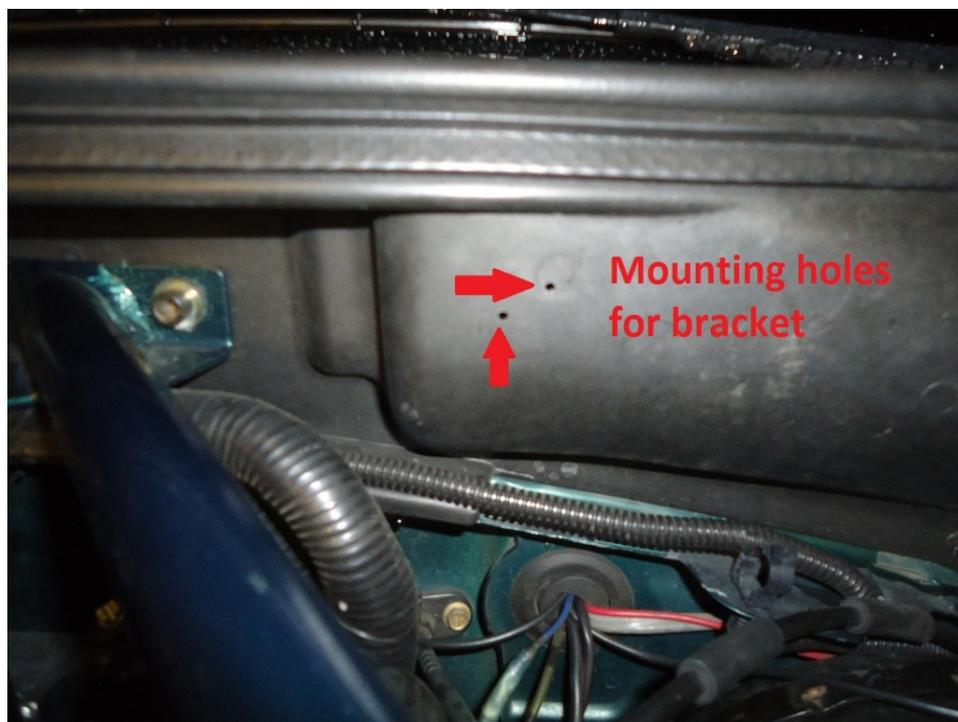
4. **For ALL models:** Drill the holes you marked with a 7/64 drill bit. You want to drill a much smaller hole because it will give the screws more material to bite into and to assure your bracket doesn't come loose.
