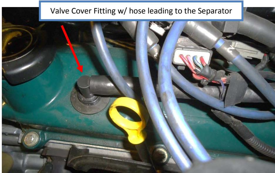
9. **For non-Cobra models:** Install the other section of hose over the intake fitting you cut earlier. Reinstall the intake manifold fitting with new hose and run it over to the left side of your separator. Trim excess if needed.
