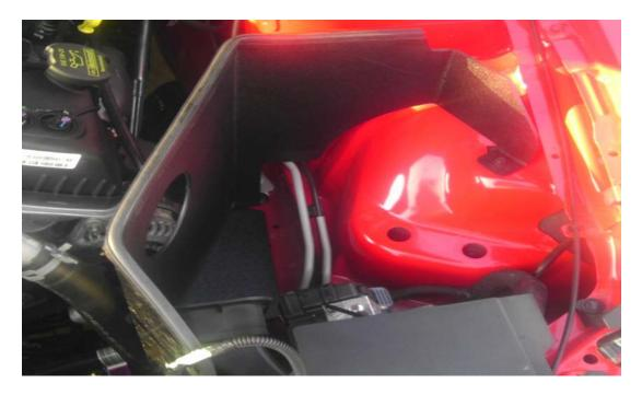
6. Place the reduction coupler on the throttle body with two clamps. Slide the JLT tube through the heat shield and insert it in the reduction coupler. Tighten the clamps **being sure not to over tighten**.
