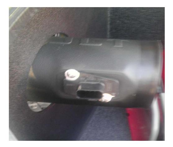
8. Install the filter at the end of the tube, making sure the clamp on the filter is loose enough to make it easy to instal. Tighten the clamp once you have it in position, **making sure not to over tighten**. Connect your Mass airflow sensor and your PCV hose.
