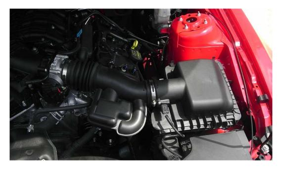
2. Locate and remove the mass airflow sensor and PCV hose from the stock airbox.
