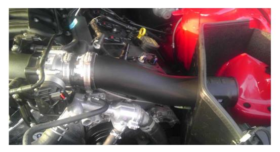
7. Remove the Mass airflow sensor from the factory airbox using the T-20 torx driver and install it on the JLT tube using the screws provided. It will only install in one position.
