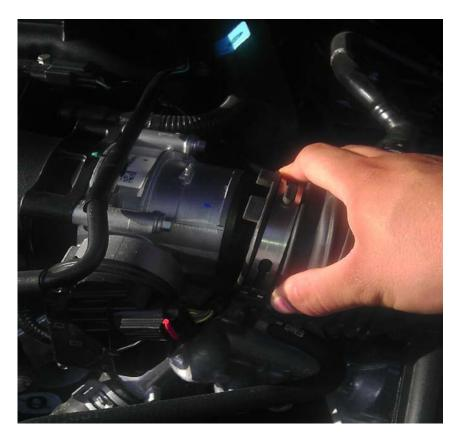
4. Using a 10mm socket remove the screw at the end of the airbox. You will then be able to remove the entire unit by lifting up.
