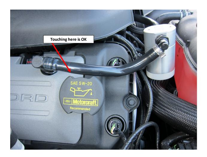
• The oil canister should be above any radiator hoses, and be well clear of the coolant reservoir, as shown here:
