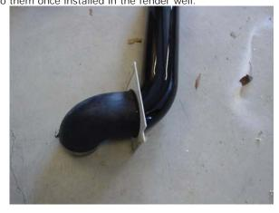
Install the MAF into the end of the reducer. Position the plug so it will be pointing toward the driver's fender and the 9 top toward the rear of the car.
