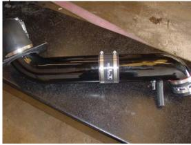
8 Slide the Apron Plate onto the pipe as if it were mounted to the apron. Next install the 90° Rubber Reducing Elbow onto the pipe.
