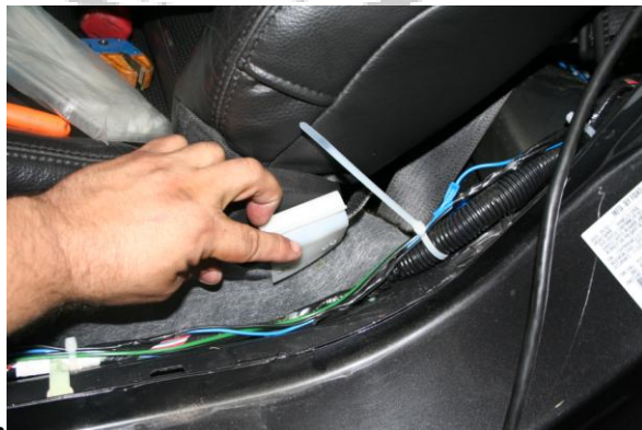
67. This is the Drivers qtr. Run the wiring using tie straps and joining them so they Run under the Drivers side door sill.
