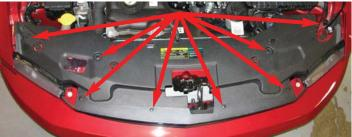
5. Use an 8mm socket to remove the two upper fascia bolts located between the grille and headlights.
