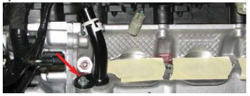
35. Use a soft cloth to remove any contaminants on the sealing surfaces of the cylinder heads. Use masking tape to prevent any debris from entering the exposed ports.
