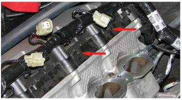
69. Mark the actuator rod where it goes into the actuator body so that it can be reinstalled in the same position, then unbolt the actuator from the manifold.
