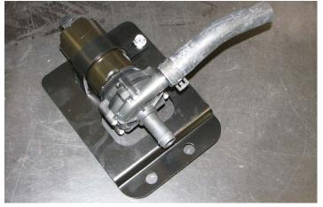
42. Fit the short molded hose onto the outlet of the water pump and secure it with a hose clamp.
