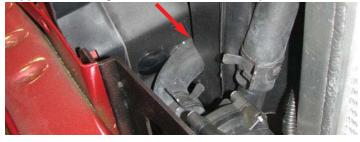
46. Install the long 3/4" hose onto the driver side barb of the heat exchanger and secure it with a clamp. Route the rest of the hose around the A/C hard line, avoiding close proximity to the exhaust manifold and power steering pump, and up between the engine and driver side fender.
