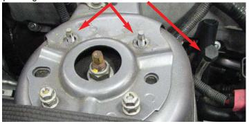
92. Remove the 10mm ground strap from the passenger side strut tower bracket and pull out the harness body pin. Route the strap to the ground stud on the outboard side of the fuse box and secure it with the nut supplied in Bag #7.
