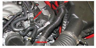
13. Use a 10mm socket to remove the bolt retaining the induction roar resonator diaphragm and lift it up to pull the induction roar resonator tube out of the firewall. Insert the grommet supplied in Bag #1 in the hole left in the firewall. Pull the tube bracket off of the strut tower and the air box.
