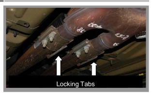
Separate the cat-back system by loosening the (2) 15mm nuts on each band clamp and prying the locking tabs up with a small flat head screwdriver while sliding the clamp towards the rear of the car.
