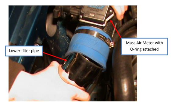
7. Tighten down all hose clamps completely at this time.
