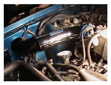
Using the image below for reference, slide the O-rings onto either side of your BBK Mass Air Meter; smaller on TB side and larger on air filter side. Slide on your (4) hose clamps and tighten down snugly so they don't fall off, but not completely using your flathead screwdriver.
