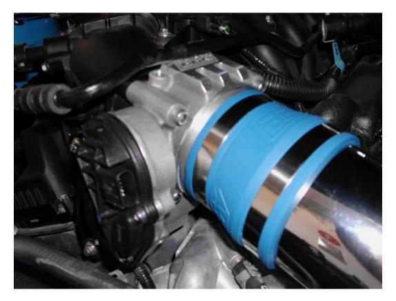
(11)A. Re-Attach the throttle body harness. Ensure the red clip in pushed back down to lock the harness in place. B. Also press the wiring harness clip back into the new throttle body.
