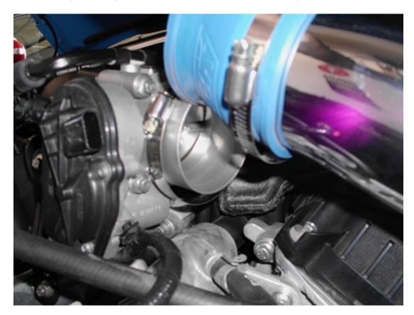
(6) You can now loosen and remove the four bolts that connect the stock throttle body to the intake manifold. For this you will need an 8mm wrench and / or socket with ratchet.
