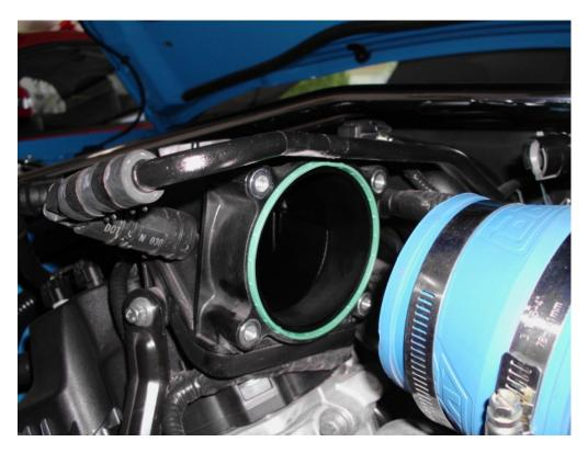
(8) Align the four bolt holes on the new throttle body with the inserts on the intake manifold. There are four new bolts supplied with the Throttle body kit from BBK. These will require a 5mm Allen wrench to tighten them. (Note: the installation instructions from BBK says that the bolts are 4mm; not sure why these were 5mm)
