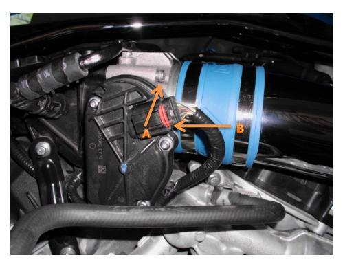
(12)Reconnect the two breather air lines on the cold air intake. Installation is complete.
