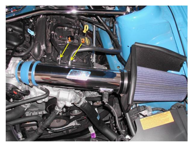
(2) Disconnect the wiring harness from the OEM throttle body by first pulling up on the red slide so that clicks open. Then firmly press against the side of the throttle body with your thumb, while pull back to pull the wiring harness free.
