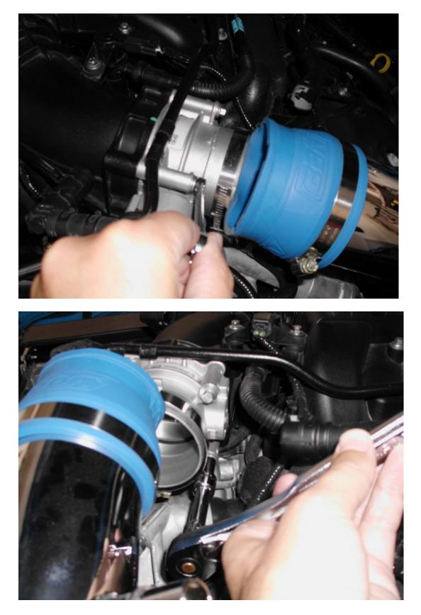
(7) Once you have removed all four bolts, the throttle body will be free. Safely place the OEM throttle body to the side. Ensure that the stock blue-green seal that is between the throttle body and the intake manifold is clean and is in good condition. It will need to stay in place for the new, BBK throttle body.
