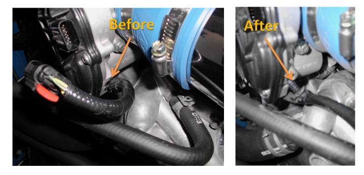
(4) A. Loosen the hose clamp(s) connecting the Cold Air Intake to the Throttle Body. (Note: There may only be one hose clamp on an OEM CAI) B. Remove the tape holding the sensor line to the top of the Throttle Body.
