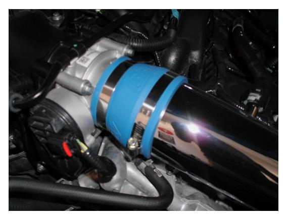
(5) Once the hose clamp is loose, pull back on the Cold air intake sleeve to separate it from the throttle body.
