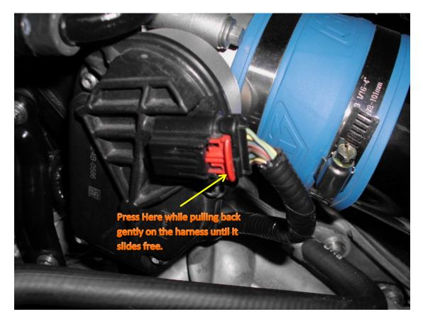
(3) In order to separate the wiring harness from the Throttle Body, gently pry the press-in connector attached to the wiring harness from the throttle body. A small screw driver and needle nose pliers will be helpful.
