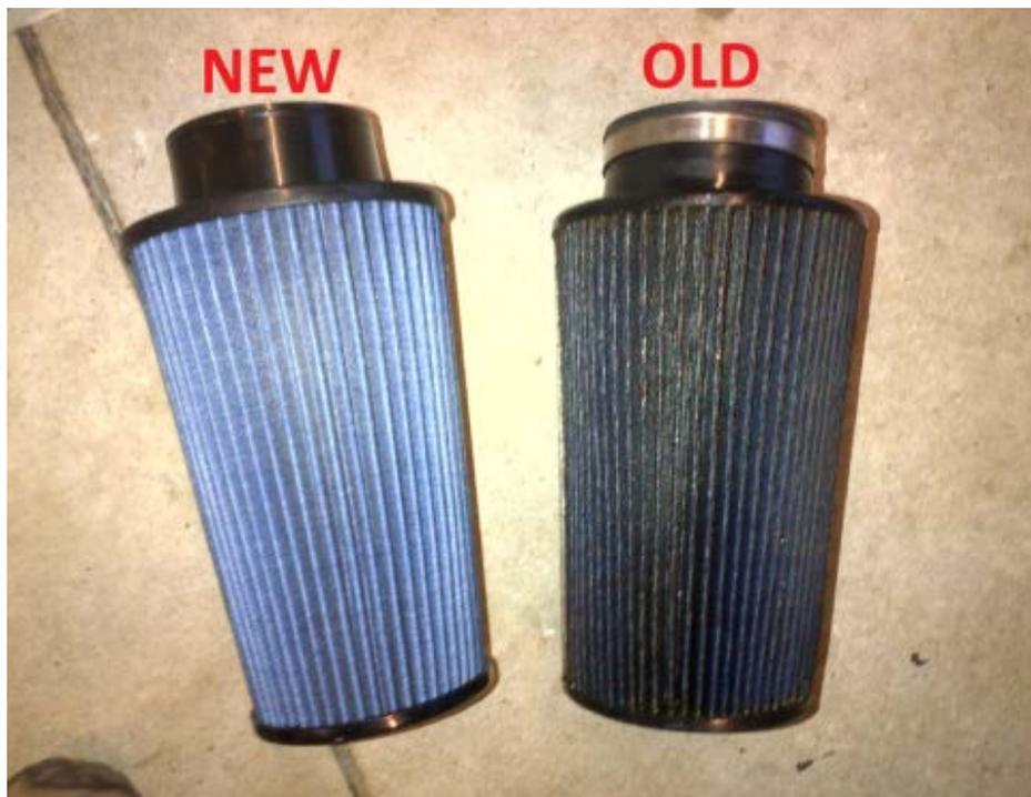
7. Carefully slide the new filter onto the air intake – make sure you place the clamp loosely over the filter first. Using a slotted screwdriver, tighten the clamp to secure the filter to the air intake.
