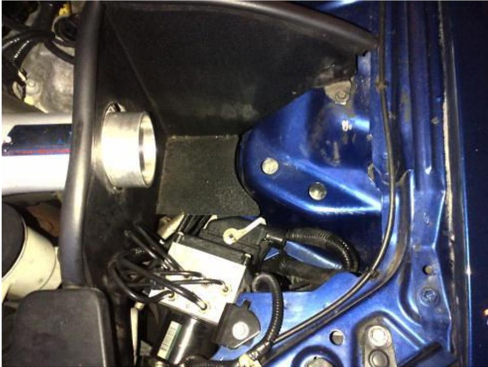
4. Also, take this opportunity to check inside the air intake. Check for dirt, debris, etc... If there is anything, clean out the air intake thoroughly. You may wish to remove your entire cold air intake (if its dirty) and clean it as this is the air that is going into your engine.
