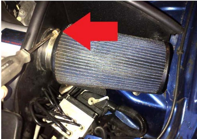
2. Once the clamp is loosened, then carefully remove the filter. You may need to move it around a bit to get it off.
