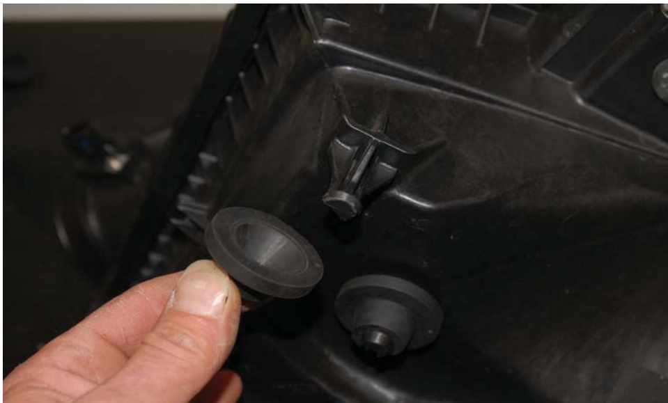
Fig. 2 Remove rubber grommets from stock air box.
