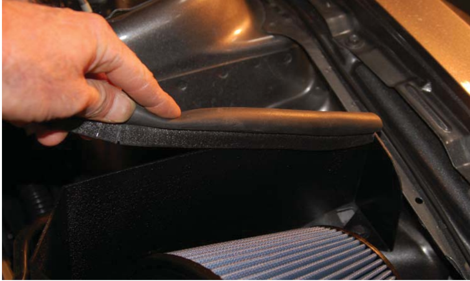
Fig. 7 Installing sponge seal to top of filter shield.
