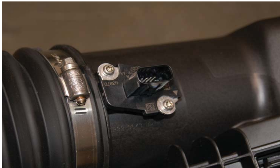
Fig. 6 Remove Mass Air Sensor from air box cover. Use a Torx T20 screwdriver.
