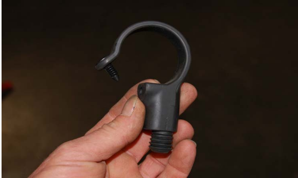
FIG. 5 Sound tube clamp. Install in the 5/8" hole on bottom of BBK filter shield.
