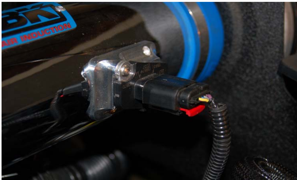
FIG. 10 Stock Mass Air Meter shown installed and plug connected. Sensor will only mount the right way.
