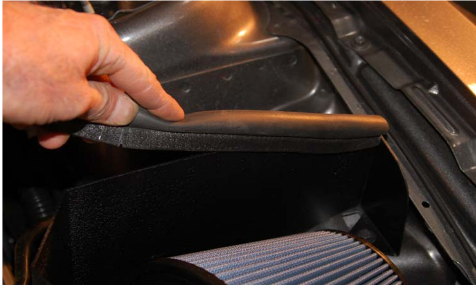
FIG. 11 Install sponge seal to top edge. Trim off any extra material.
