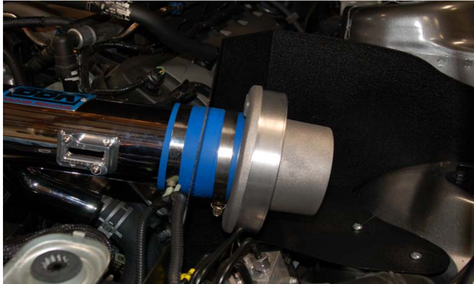
FIG. 9 Cast aluminum filter adapter shown installed.
