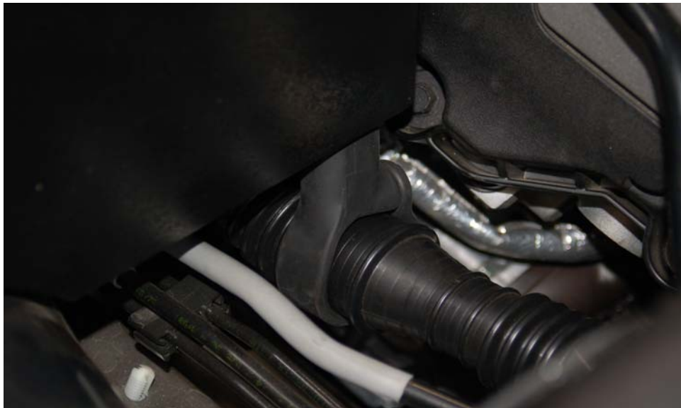
FIG. 6 Sound tube clamp installed and holding sound tube that now runs under the filter shield.
