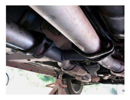
**Step 5.** Slide the hangers attached to the stock H-Pipe off of the rubber mounts and completely remove the H-pipe from under the car. Set aside the stock pipe where it will be out of your way.
