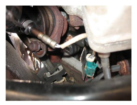
**Step 2.** Use an O2 Sensor Socket with your Ratchet or Adjustable Wrench to remove all 4 O2 Sensors from the stock H-Pipe. Once removed, set them aside in a safe location.
