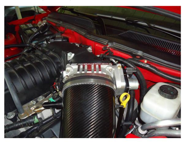
21. Attach the MAF connector to the inlet tube and press in the red tab to lock it in place. If you installed an aftermarket CAI, you will need to transfer the MAF Sensor from your OEM tube to your new tube.
