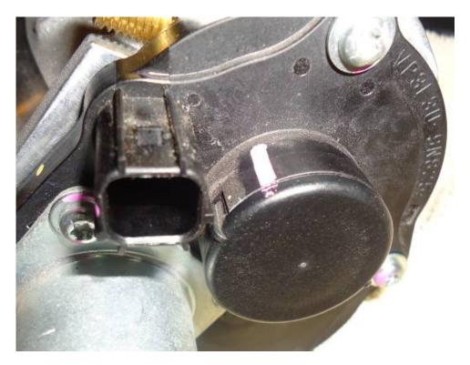
18. Install the new TB onto your intake elbow. Use the 2 shorter bolts that were supplied with the TB on top; use your original bolts on the bottom. The top bolts require a 5mm Allen wrench.
