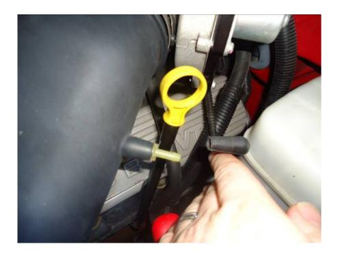
6. Use the large flathead screwdriver to loosen the hose clamp at the throttle body. Remove the airbox (or CAI) and inlet tube from the car using a flat blade screw driver.
