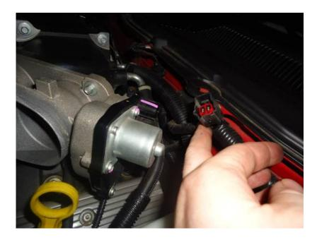
8. Use your 5/16" socket to remove the 4 bolts holding the throttle body to the intake elbow. You'll need to use the extension on the lower bolts. Be sure to hold the throttle body with one hand before you remove the last bolt so it doesn't fall.
