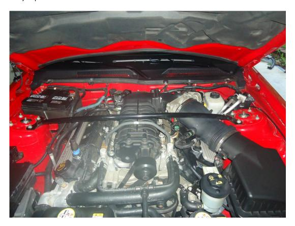
4. If you have an aftermarket CAI, remove it from your fender. If you have the stock airbox, use the 13/32" socket to remove the bolt holding it to your fender. On the MAF Sensor connector, pull out the red tab and remove the connector.
