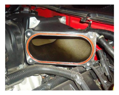
10. Now we need to transfer the TPS and Motor Housing from the old TB to the new one.
