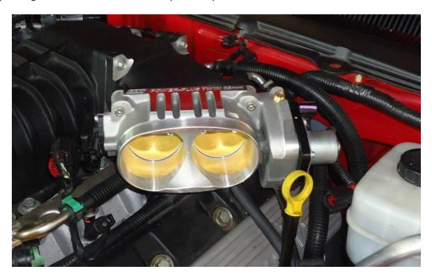
19. Reinstall the two connectors to the TB. Press in the red tabs to lock them in place.
