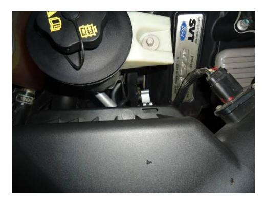
5. Gently twist the green locking tab on the PCV tube going to your inlet tube and remove it. Gently pull the vacuum hose from the inlet tube.
