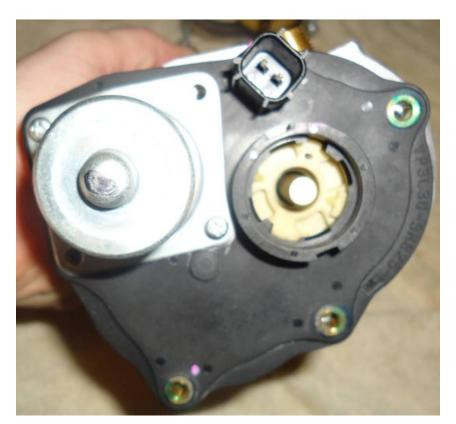
16. Firmly grasp the tan spring cap with your needle-nosed pliers. Rotate it 180° counterclockwise. This will make the indentions line up with the black tabs on the motor housing. Once they line up, pull the tan spring cap up. It should lock into place.
