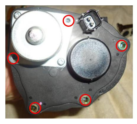
13. Flip the motor housing over. Remove the spring and set it aside. Flip it back over and use your finger to pop off the black cap from the backside.
