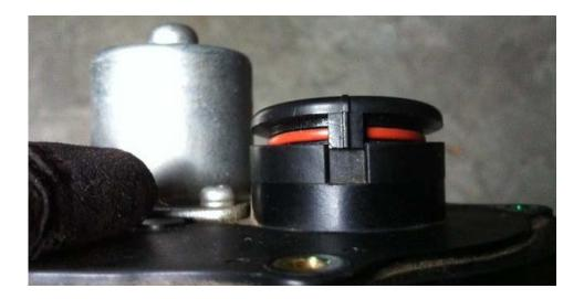
8. Place the plastic capped spring over the BBK throttle body shaft and line the pigtail hook into the catch slot. Do not place the removable cap on yet.
