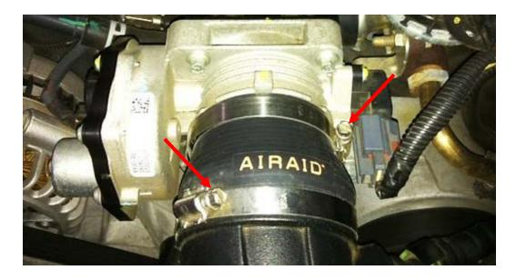
4. Unplug the throttle body electric motor and TPS wires. You can do this by sliding the red tabs back, squeezing the grey tabs that will be exposed and pulling back carefully.
