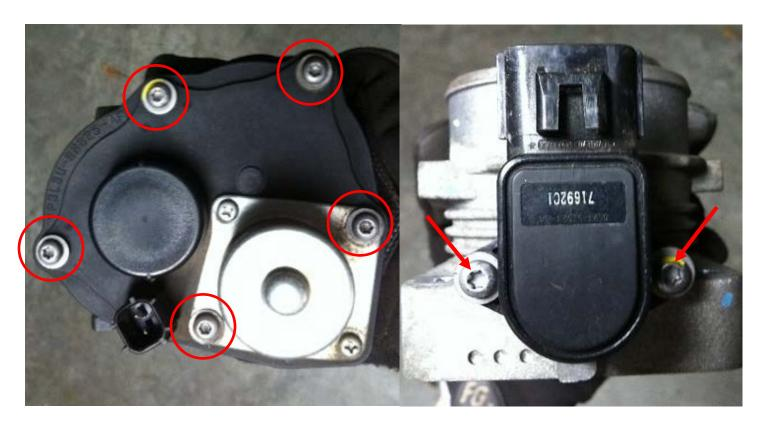
7. Using a screwdriver, gently pop the circular cap off the motor housing.
