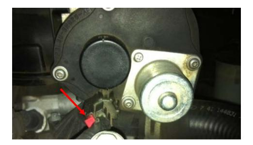
**2005 V6 ONLY:** If you have the (2) coolant hoses that route through the stock throttle body, disconnect the hoses and bypass them, clamping down the supplied U-shaped tube.
