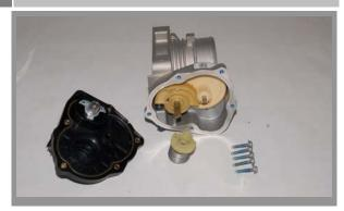
Remove the five Torq Head Screws and remove the motor cover and internal spring. Be aware that the cover will want to rotate as the screws are removed because of the internal spring being under some tension.
