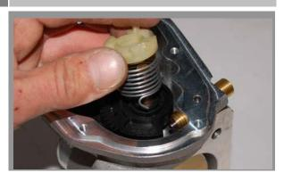
Install the internal spring on the gear in the BBK Throttle Body. Make sure the hook on the end of the spring is in its mounting hole in the gear.
