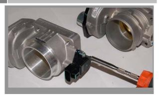
Remove the TPS sensor and re-install on the BBK Throttle Body using the stock screws.
