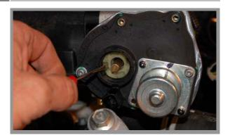
Using your small screwdriver, push in on the white spring retainer to release the spring. Unplug and remove the motor cover. Tighten the set screw for the brass adjuster stud. Reinstall the motor cover, reclock the internal spring counter-clockwise and lock the tabs into place. Reinstall the round plastic cover. Plug in the motor control wires.
