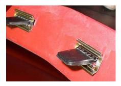
STEP 6: Use a drill and a 3/16" drill bit to drill a hole through the bottom of the grille and into the top of the front fascia. The hole should be located between the two center tabs and as far forward as possible. Once the hole is drilled, install the one push tree clip provided. The tree will be used to secure the bottom to the grille to the top of the fascia.
