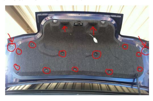
Once the trunk liner is removed you will then notice four (4) nuts that will need to be removed. They are all the same size and can each be removed using your 10mm socket. The nuts under the rubber grommets will be labeled below as (A) and the same bolts, just under the trunk liner, will be labeled as (B). They will all be highly recognizable once the trunk liner and grommets are removed.
