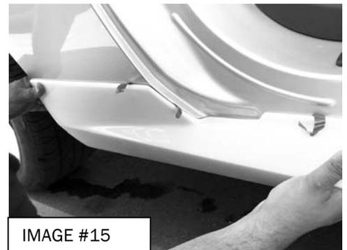
Step 7) Using the supplied #8 x 3/4" self-tapping screws, secure the side skirt in the wheel wells through the pre-drilled holes in the rear of the side skirt. Using the factory clips removed from the original side skirts, secure the front of the side skirt through the pre-drilled holes.
