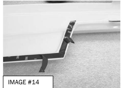
Step 6) Place the side skirt on the car, positioning it using the grease pencil marks as a reference. Starting with either end, pull the red backing tail and press the new side skirt to the paint surface at the same time. (See Image #15)
