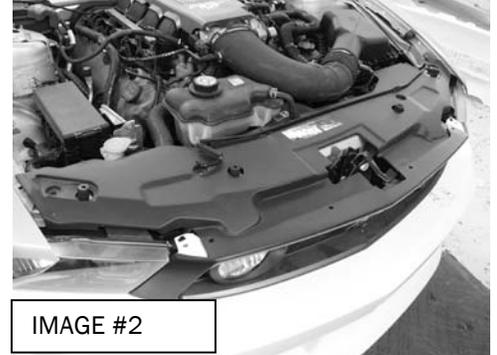
STEP 2) Carefully pull the bumper forward enough to access the wiring connectors on the side fog and marker lights. Disconnect the plug from the side marker lights. Locate and remove the air temperature sensor and relocate it as shown in images #3-5. Now remove the bumper completely from the car. Remove the front marker lights and the front grille from the bumper.
