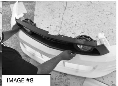
STEP 5) Lay the new 3d bumper replacement upside down. Place the supplied aluminum mesh grille inside the bumper. Check fit the grille in the opening. Using a screw gun with a Phillips head tip and the (6) stainless steel screws and washers provided, secure the aluminum grille to the front bumper. (See Images #9-10)
