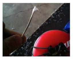
7. Use the greased Q tip to get inside the new distributor boot on the new wires and apply a thin layer evenly on the inside.
