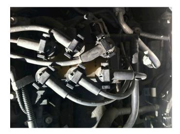
2. Follow the wires along to the boots and remove any of the factory wire clips. Use the flat head driver to pop the clip apart.
