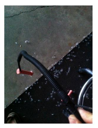
9. Once all new wires are prepped to go on, remove one at a time the factory boots from plug and using old wire, compare with new wires and find the wire that closest matches the length. Install the wire onto the coil pack by putting the brass end in first then pushing down until clasps close around base, run the wire to the appropriate plug and push new boot on until a pop or click noise is heard. Make sure wire isn't resting on anything that will get extremely hot.
