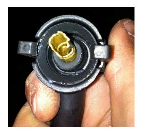
Similar to step 7. Apply grease with Q tip to the inside of the new plug boots. <u>DO NOT</u> go all the way down to metal, only grease the rubber part.
