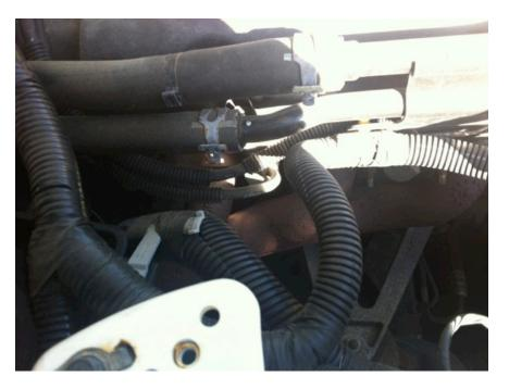
4. Remove each of the old spark plug wires by squeezing tabs and lifting off from the old coil pack. A little force will need to be applied. Also twist while pulling if they are being difficult.
