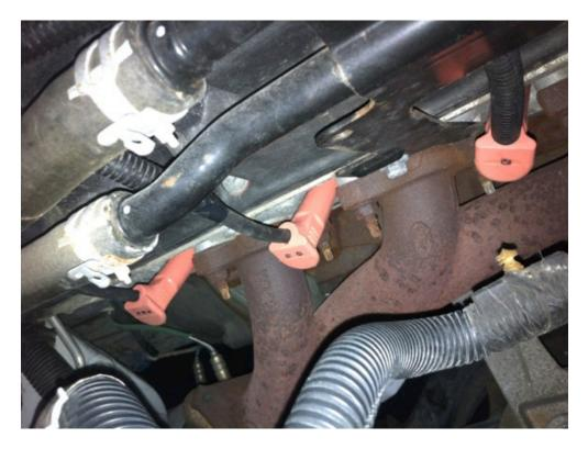
10. Once all boots are seated on plugs and pop is heard. Check to make sure all wires are not in danger of heat damage. Re install the factory 3 wire clips onto wires where ever they dangle loose.
