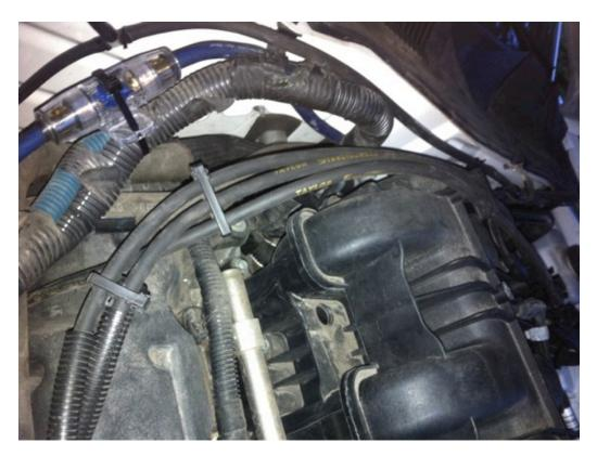
3. You need to now unplug the wires from the spark plugs, this includes pulling and wiggling. They have stronger boots around the ends that you can grab to help you pull the spark plug out.
