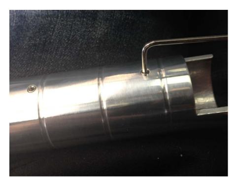
5. Then drop the button in and hold on to it from the outside while sliding the handle over your existing handle. (this will be a tight fit but with some twisting it will go all the way down)
