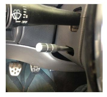
8. For the turn signal cover, loosen the one screw with your supplied allen and place it over your turn signal then tighten down the screw. Do not over tighten, keep in mind its plastic underneath.
