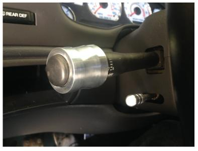
9. Finally the last thing to do is your headlight knob. Start by pulling it out as if turning on your headlights and turning it so that the slot faces out.
