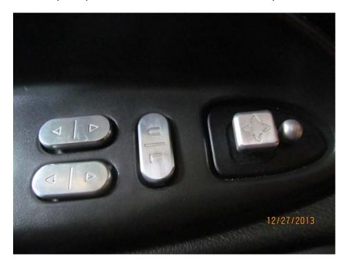
5. The electric mirror knobs pry off the same way. There is a rubber spacer that is included with the factory knob. I used it with the new Billet knob (see photo below of spacer).
