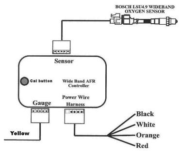
Parts included: Bosch LSU4.9 Oxygen Sensor Sensor wiring harness Weld in bung
