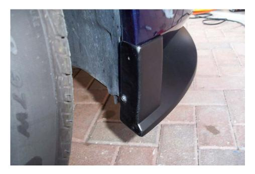
7. The spoiler is now installed using the tape. Now you will need to finish the installation with the screws provided by Stillen. Start by drilling holes in the bottom of the bumper that line up with the holes in the Stillen Chin Spoiler; there are (5) of them.
