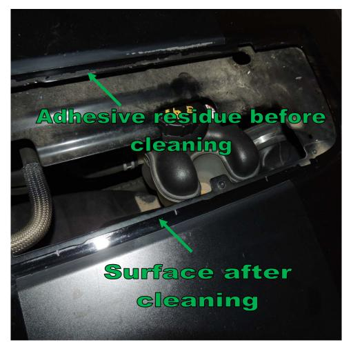
14. Thoroughly clean the hood cut-out. Wipe the area down with Isopropyl Alcohol and allow to evaporate so that no contaminants remain. This hood has been cleaned, restriped, and cleaned again in preparation for the new heat extractor.
