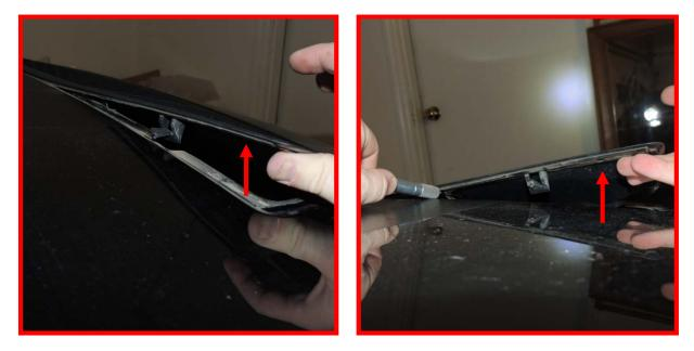
8. Continue to pull up on the driver side, carefully using the precision knife to cut the adhesive tape as you go. Again, stop before you reach the center stud (which had the nut on it from Step 4).
