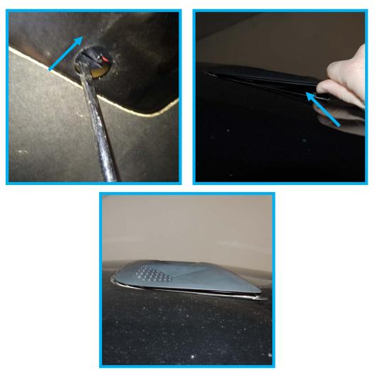
7. Continue to pull up on the passenger side, carefully using the precision knife to cut the adhesive tape as you go. Stop before you reach the center stud (which had the nut on it from Step 4). You can see I broke the tab on this side by not performing Step 5 correctly.
