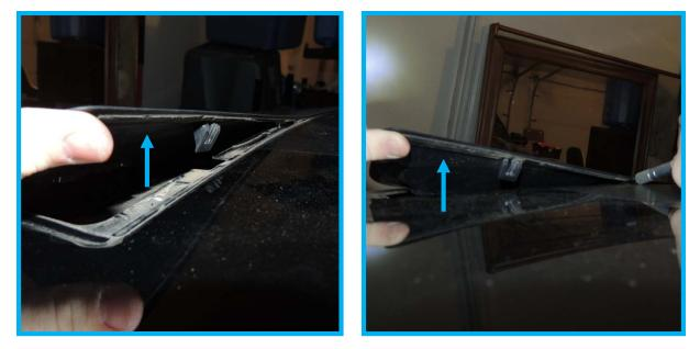
9. Now, you should be able to easily lift the rear of the heat extractor off of the hood. Pull the piece towards the rear of the car and it should slide out.
