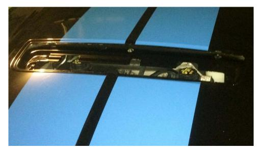
15. Inside the front edge of the new extractor, there is a center alignment tab.
