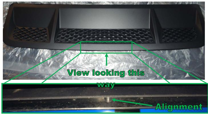
16. This tab fits perfectly into the center slot in the forward edge of the hood cutout.
