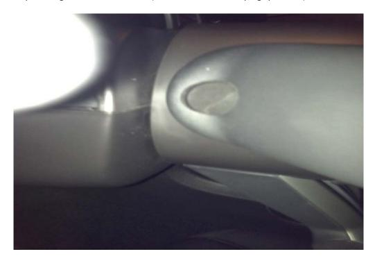
3. Using the 8mm socket and extension to easily remove the bolts on each side of the steering wheel. Save both bolts you will reuse them. (Bolts showed removed in picture below)
