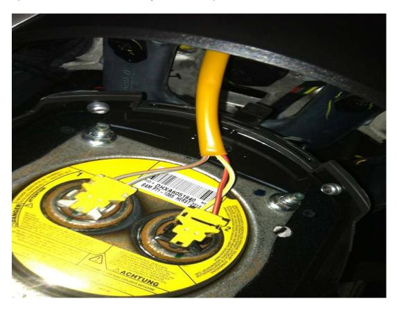
5. After that unplug the cruise control plug and then unbolt the 24mm bolt in the center of the steering wheel using socket and extension so that you do not scratch the steering wheel. ( the plug is beside the yellow cable and the bolt is shown below)
