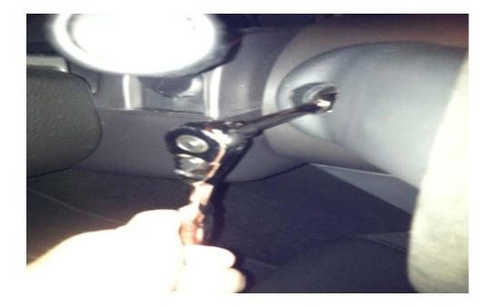
4. Next pull the airbag module out with both hands on each side (Not to far though because the 2 electrical cords don't pull out far). After the module is out pinch the side of the tabs and pull up. (tabs on the back of the module pictured below)
