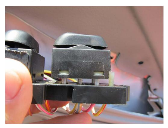
7. Take your new switch, and just plug it into the now vacant spot. At this point, you might want to turn your accessories on, and make sure the switch works. It should work perfectly fine, and if it does, you can continue with putting the switch back into its bezel, and securing it in place with the screws.
