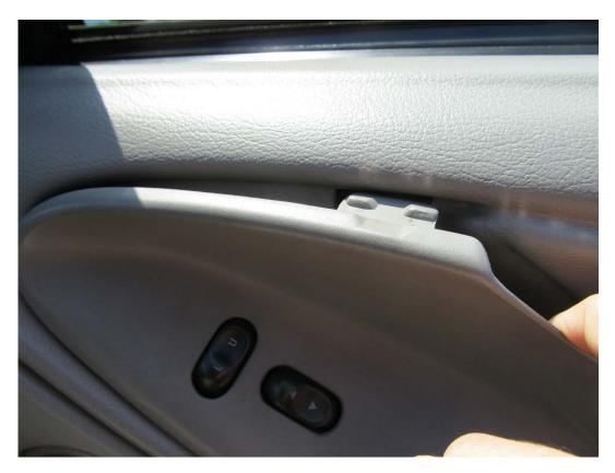
3. Now, on the bottom left hand side, pull this side upwards towards the window, it should pop up easily.
