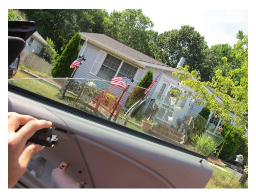
8. Once everything is in working order, secure the board to the bezel with the screws, and then put it back in reverse from how you took it out. (Make sure the clip is on the tab!) Take the bottom right corner, and gently push that in. Now, take the bottom left corner and push that in, and the top most clip should just slide into place. Everything should be working fine now. Enjoy having the windows down!
