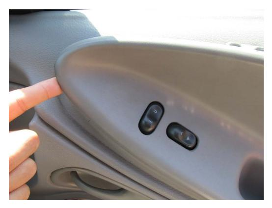
4. Lastly, you can now pull up the bottom right hand side. Be careful as this one will be a little stuck in there, you must carefully grasp the entire bezel and pull it upwards. As long as the clip is still attached, there should be no problems. If the clip falls off, just put it back on the plastic tab so if it needs to be removed again, the tab will not crack. If you are missing your clip or it is broken, you NEED to order another set as it will prevent this tab from snapping.
