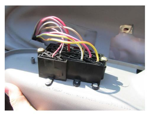
6. Now that it's removed, you should see either two switches (Passenger side) or three (Drivers side). You're going to want to gently grasp the malfunctioning power window switch, and wiggle it back and forth upwards until it starts becoming looser, and eventually pops out.
