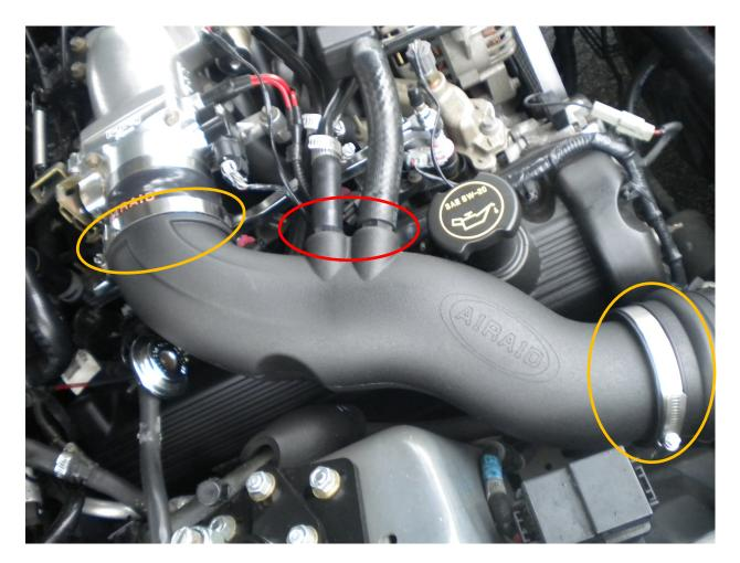
3. Locate the PCV valve, and remove the vacuum line. Carefully clean around the PCV valve with a shop rag. Using the pliers, give the PCV valve a counterclockwise twist and pull it out of the valve cover.
