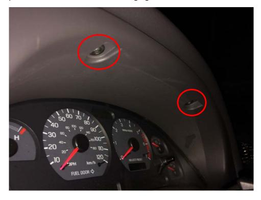
3. Once the screws are removed, carefully remove the plastic surrounding the cluster. Pull from the bottom first and when you feel it come free, wiggle it out from behind the steering wheel. Adjusting the steering wheel might help.
