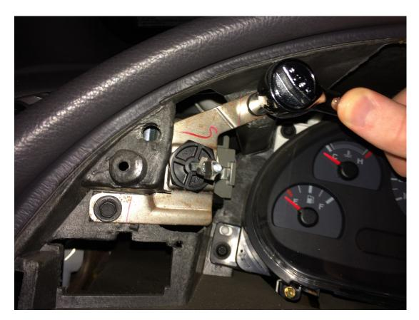
8. Replace the two screws above the gauge cluster.
