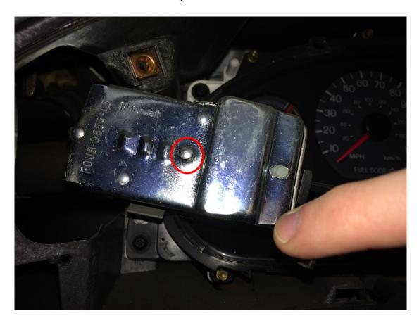
6. Put your replacement rod inside the box and it will lock in. Make sure you remove the knob or else the dash won't be able to fit back on.
