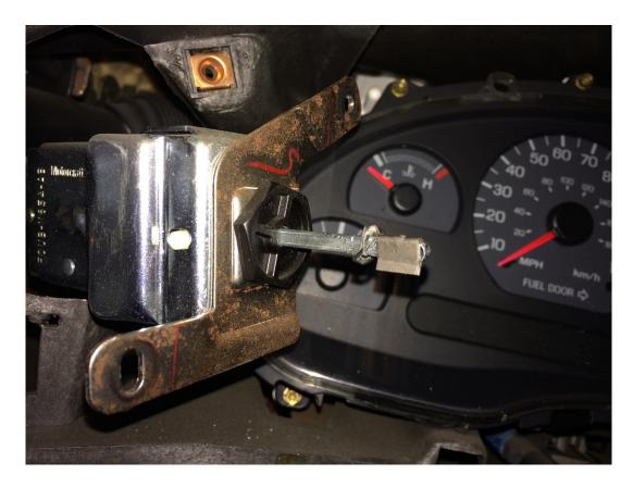
7. Replace the two bolts inside the dash.
