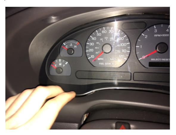
4. Next, use a 9/32 socket to remove the two bolts inside the dash.
