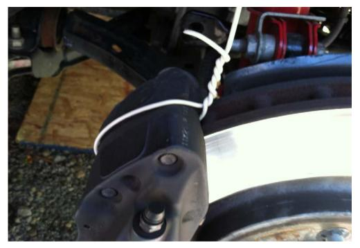
5. Now it is time remove the two caliper mounting bolts. Use the 15mm socket and breaker bar to loosen the 2 bolts then continue to remove with 15mm and ratchet wrench. The caliper will pull straight off toward the cabin of the car. The brake pads may fall to the ground as they will be loose.
