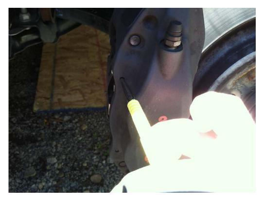
4. Once both pins and the retainer clip are removed you need to secure the caliper with wire to prevent brake line and caliper damage. I found it easiest to run the wire along the top of the rotor through the first part of caliper and then around the coil spring.
