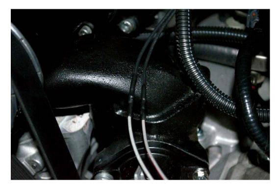
12. Once this is done, you can use some wire loom or route the wires as you please, for aesthetics. As far as the sensor is concerned, you are finished and the IAT has been successfully relocated. Start your vehicle and ensure that there are no MIL codes. You can also use an aftermarket ECU tuning device to monitor the IAT from the new sensor to ensure its working. However, if you have no MIL codes, then the ECU is getting a proper signal for your relocated IAT sensor.
