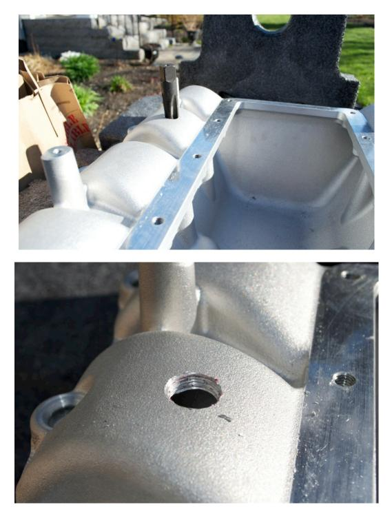
3. At this point, thread your sensor gently to test and make sure the threads work. There is a red thread locker on the sensor, it will give some resistance when you try to thread in the sensor. Just be gentle and thread past it. Clean up any residue left over on the threads (you will see it, it will be the red/pink paste).
