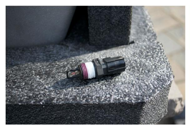
5. With the Teflon tape wrapped, thread the IAT sensor into the hole you made. Once it is hand tight, give it another 90 degree turn with your adjustable wrench. Be gentle as the sensor is plastic. Use your judgment and stop tightening if you feel a lot of resistance. The Teflon tape should do its job and create an airtight seal. (Note that this picture does not have the Teflon tape on but it should).
