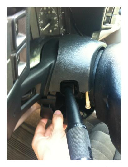
2.) Once the column is out, you should be able to remove the knee guard, but if you look on the bottom of the guard you'll find three screws which are 8mm. Take all the screws off and safely remove the knee guard to make sure you don't crack the plastic. Next will be the metal knee plate; which also has two 8mm screws holding it in place. Remove those are place plate aside.
