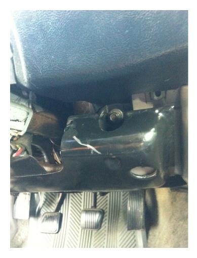
3.) When the metal plate is removed, remove the two 7mm screws from the top of the dashboard and gently remove to prevent cracks in the plastic. Next, you'll have to remove the two clips holding the headlight/foglight switch. Once that is done you, can pull the switch right out of the dashboard by unclipping it from the wiring harness.
