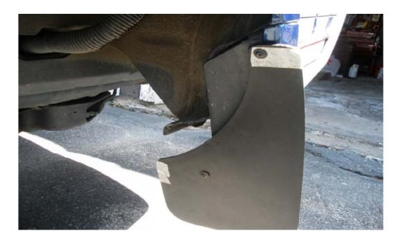
14. Only do this if your drill holes are properly aligned with the screw wells. Take the splash guard with the drilled out holes and hold it against the other splash so that they are aligned together. Then clamp them at two points as shown in the picture below.
