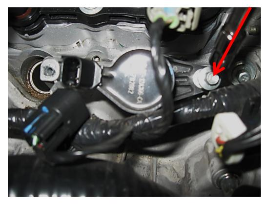
**Step 6:** Gently pull straight up on the assembly and lightly wiggle left to right to help release the seal and it should come right out. Now, blow out the spark plug ports with compressed air.
