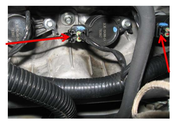
**Step 5:** Remove the 7mm bolt which is located to the right of each coil pack, (8) total bolts.
