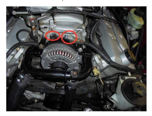
if you took the water pump pulley off reinstall that now, use a breaker bar or ratchet to put tension on the belt tensioner and reinstall the serpentine belt onto the alternator and pulleys.re tighten the water pump bolts. Check the belt make sure its on correctly and Reconnect the negative battery cable, start up you're car and enjoy the new 130 amp alternator
