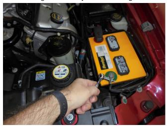
2) go ahead and use a flathead screwdriver to gently push the tab on the electrical connector out (towards the windshield) and lift the connector up and out of the way.
