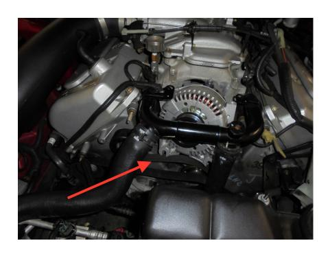
8)now just reverse the process re install the (6) bolts with you're 10mm socket, reconnect the two electrical connections on the top as shown.
