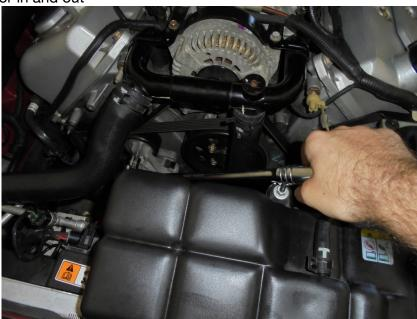
5) now with belt out of the way you can use a 10mm socket to remove the (6) bolts holding the alternator in place.(2) bolts on the bottom front and (4)bolts on the top
