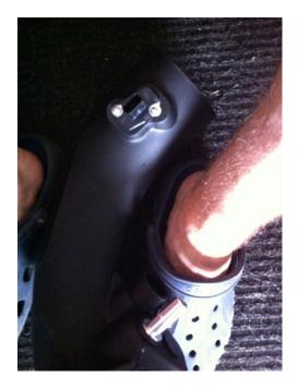
5. Once all pieces are attached to the intake tube, attach the tappered rubber grommet to the front of the tube with the medium sized hose clamp. Then attach the last grommet with the bubble in the middle to the end of the tube with a large clamp. After that secure the tappered grommet to the throttle body with a small clamp. (soapy water helps get hose and grommets together)
