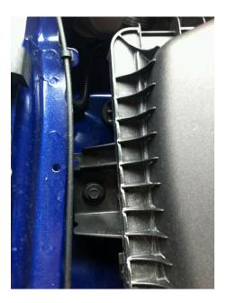
3. Once you have taken the stock airbox intake system off, assembly of the Airaid intake is next. Start by securing the new heat shield into the car in place of the old airbox. Use the 10 mm socket on this again to put bolt back into the same hole.
