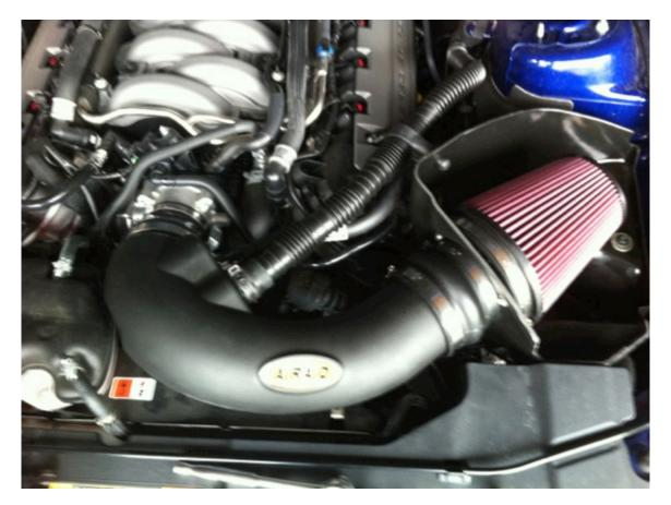
8. Put the plenum back into the engine and reattach the strut tower brace. Double check that everything is tight. And enjoy the power and sound you get from your new Airaid Cold Air Intake!
