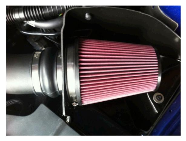
7. Once all tubes and clamps and grommets are in the correct place. Proceed to use the 8mm socket or flathead to tighten all of the clamps so that nothing with come loose from the pressure. Reattach the mass air sensor, vac line and sound tube to the new intake tube using the pliers and soapy water.
