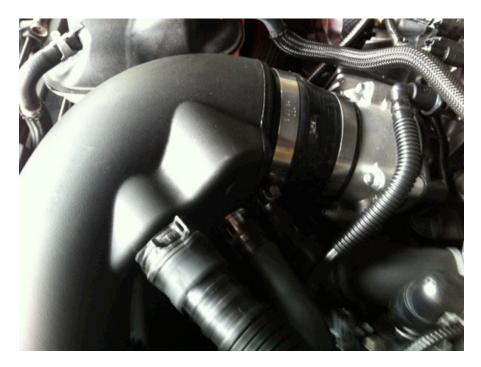
6. After securing the tube to the throttle body, attach the end of the tube with the big grommet to the other grommet that we secured to the heat shield using another large clamp. After that attach the air filter inside the heat shield with the last biggest clamp.
