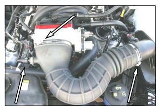
5. Reinstall the intake tube, and tighten the hose clamps. Reconnect the breather hose to the intake tube. 6. Inspect & test the throttle linkage for full open and closed travel before driving. Some cruise and kickdown cables may require adjustment. Please refer to vehicles service manual for proper adjustment.
